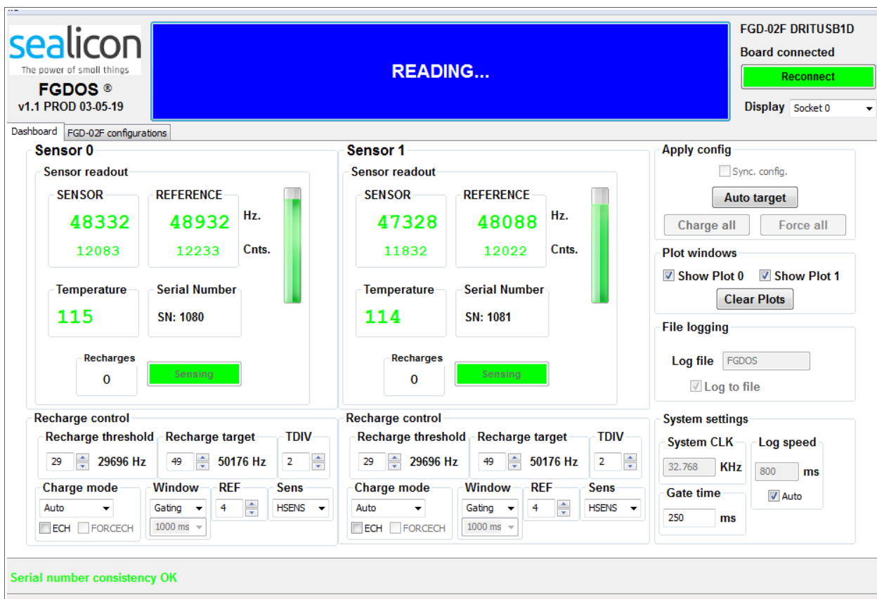
Figure 6. Default view of the GUI for controlling FGD-03F_Z1 sensors with Dashboard panel selected
